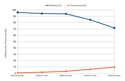
Air flow  $[m^3/h]\,/$  Speed air trought the filter [m/s]
