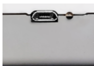
USB type B - power supply
