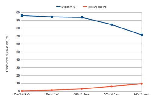
Air flow [m³/h] / Speed air trought the filter [m/s]
